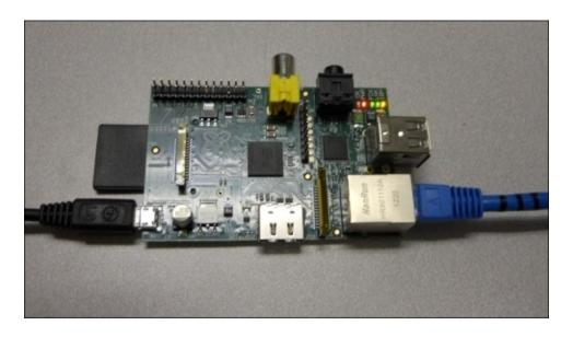
You need to connect the power and LAN. If you need to issue simple commands, you can connect via SSH. If you need a more complete set of graphical functionalities, you can access them via vncserver. Finally, if you are using a Windows system and want to transfer files back and forth, you need access to WinSCP. Now you have the toolkit to build your first set of capabilities.
