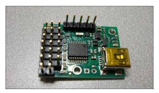
Make sure you order the assembled version. This piece of hardware will turn USB commands into voltage levels that control your servo motors. Pololu makes a number of different versions of this controller, each able to control a certain number of servos. Once you've chosen your legged platform, simply count the number of servos you need to control and choose a controller that can control that many servos. In this book, we
