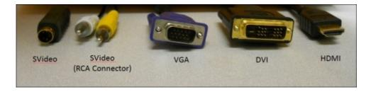
There is an SVideo output and an HDMI connector on Raspberry Pi. The easiest method to create a connection is to connect the board directly to a monitor or TV that has an SVideo or HDMI input; however, you'll need to buy a cable to go between the two. Check the video input on the monitor or TV; it will normally either have a set of RCA jack inputs, normally colored yellow (video), white (left-audio), and red (right-audio), or a multipin SVideo connector. If you are connecting using the RCA jack
