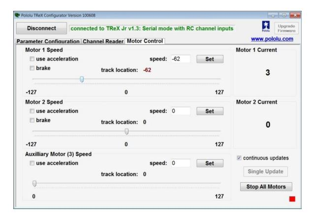
The motor should now be running! You have control of the DC motor. Now connect the second motor, repeating the connection steps detailed earlier in this chapter. Now you should be able to control the speed of both Motor 1 and Motor 2.
