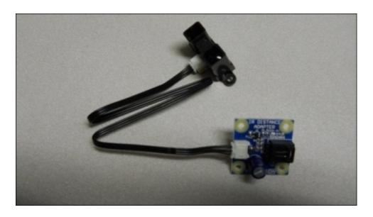
2. Now, you need to connect the IR Distance Adapter to the USB interface board. Connect the board using two cables, as shown in the following image (fortunately, there is only one way to connect them):
