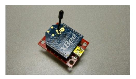
As noted at the beginning of this chapter, you will be learning how to use this specific device. The advantage of using this device is that it is configured to make it very easy to create and manage a simple link between two XBee Series 1 devices. Make sure you have an XBee device that supports ZigBee Series 1. You'll also need to purchase a shield that provides a USB port connection to the device.
