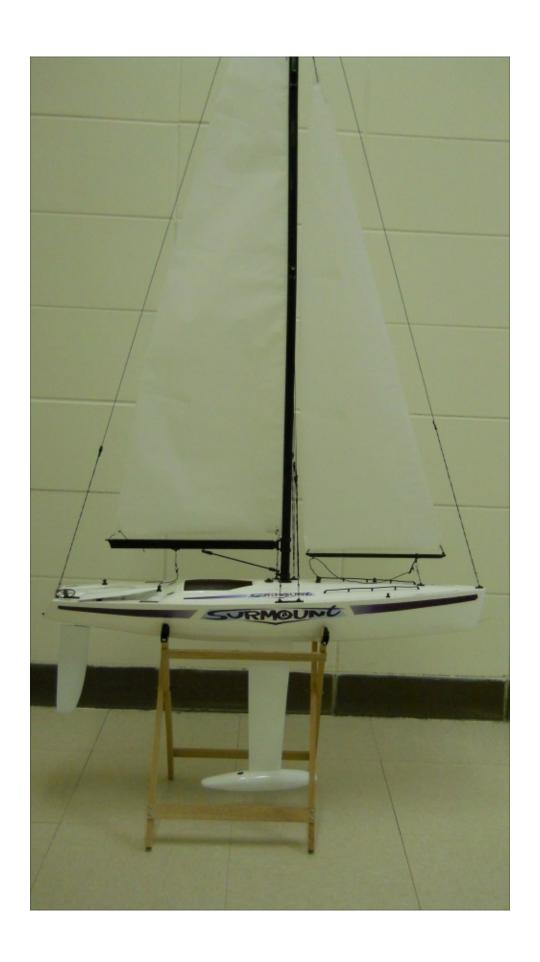
In fact, many RC-controlled boats can be modified to add Raspberry Pi. All you need is space to put the processor, the battery, and any additional control circuitry. In this case, the sailing platform has two controls: a rudder, which is controlled by a servo, and a second servo, which controls the position of the sail, as shown in the following image:
