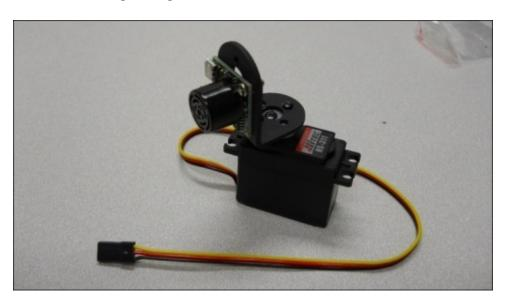
However, if you want to get really fancy, you can purchase a **Pan and Tilt assembly**. This contains two servos and allows you to rotate your sensor in both the vertical and horizontal axes. The assembly is available on online stores such as <a href="https://www.robotshop.com">www.robotshop.com</a>. You can also construct a Pan and Tilt assembly out of the components that you may have if you have purchased a legged robot kit.
