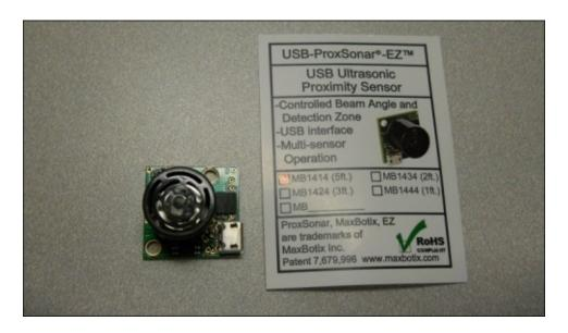
This is the **USB-ProxSonar-EZ** sensor, which can be purchased directly from MaxBotix or on Amazon. There are several models, each with a different distance specification; however, they all work in the same way.
