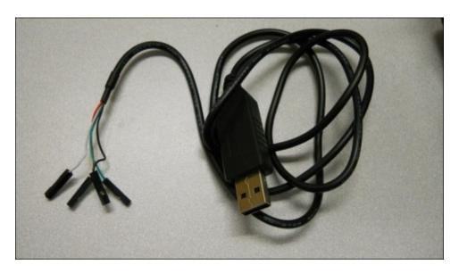
The red and black wires are for connection to the power. These can be connected to the servo controller in the following manner:
