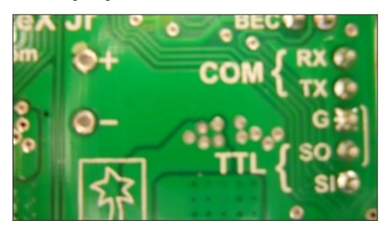
3. Now connect the green cable to the SI connection, the white cable to the SO connection, and the black cable to the G connection. The following is an image of what this should look like:
