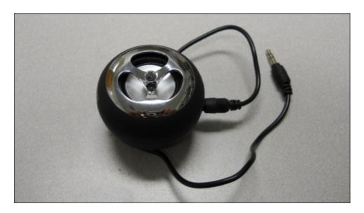
Fortunately, these devices are very inexpensive and widely available. Make sure the speaker is powered because your board will generally not be able to drive a passive speaker with enough power for your applications. The speaker can use either internal battery power or an externally powered USB hub. Many of your robotics projects will require a powered USB hub, so it's a good investment.
