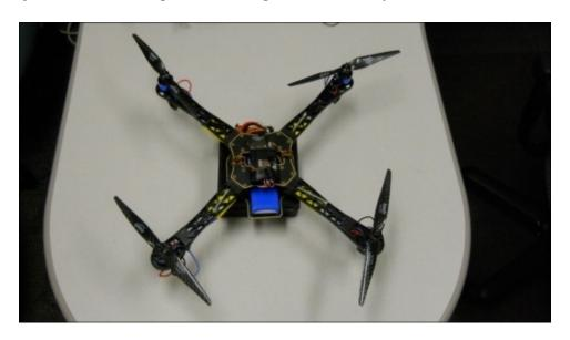
The quadcopter has two sets of counter-rotating propellers; this simply means that two of the propellers rotate one way while the other two rotate the other way to provide thrust in the same direction. This provides a platform that is inherently stable. Controlling the thrust on all four motors allows you to change the pitch, roll, and yaw of the device. The following figure may be helpful to understand the same:
