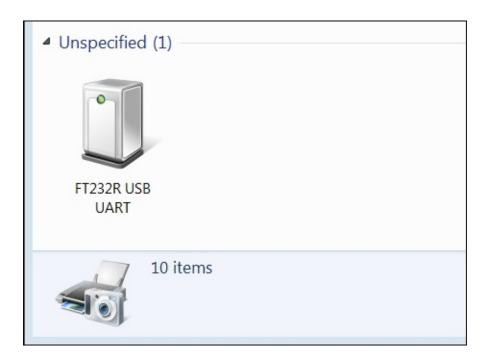
The device is now available to communicate with via the IEEE 802.15.4 wireless interface. We could set up a full ZigBee compliant network, but we're just going to communicate from one device to another directly, so we'll just use the device as a serial port connection. Double-click on the device icon and then select the **Hardware** tab; you should see the following screenshot:
