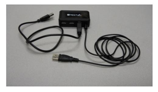
Notice that there are two connections on this hub. The one to the far right is a power connection, and it will be plugged into a battery with a USB port. The connection to the left is the USB connection, which will be plugged into Raspberry Pi.
