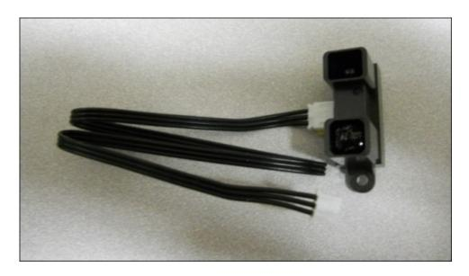
The second part that you'll need is an IR distance adapter, which can provide the signals to the sensor and condition the signals coming back from the sensor. The model number is **1101\_0 - IR Distance Adapter**. The following is an image of it:
