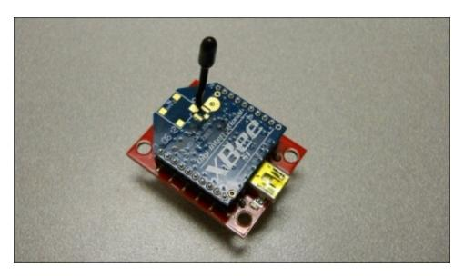
This is the device we will use in this chapter. Make sure you purchase an XBee Series 1 device as it is the easiest device to configure and use, and there is a great open source community support for the device too. If you choose a different device, you'll need to follow the directions for that device from the manufacturer. Also, if you want to use this type of point-to-point communications, you'll need two units, one for Raspberry Pi and the other for the host computer.
